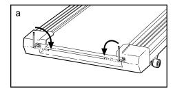
b. If the walking belt has shifted to the right, first remove the key and UNPLUG THE POWER CORD. Using the allen wrench, turn the left rear roller adjustment bolt counterclockwise, and the right bolt clockwise, 1/4 of a turn each. Be careful not to overtighten the walking belt. Plug in the power cord, insert the key and run the treadmill for a few minutes. Repeat until the walking belt is centered.
